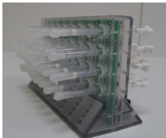
Fig. 1. Actimeter for testing male motility. The DAM actimeter is a monitor made up of a grid pierced with 32 holes. A  $65 \times 5$  mm polycarbonate tube (5 mm i.d.) is inserted into each hole, which is equipped with an infrared photoelectric detector. This configuration allows for automatic, continuous, and simultaneous recording of the displacements of 32 individuals. At one end of the tube, standard corn-meal medium was inserted and the tube was closed with paraffin.
